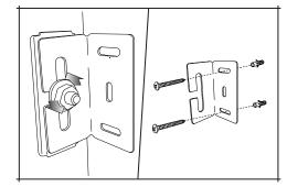
To remove the doors simply open the door and press the button at the back of both hinges.
