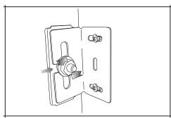
Locate the plates on the inside walls of the unit onto the wall mounting plates. Secure the unit to the wall by tightening the screw. Use a spirit level to ensure the unit is balances horizontally.
